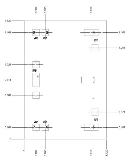
Unit: millimeters Thickness: 0.10 Die x, y size tolerance: +/- 0.050 Chip edge to bond pad dimensions is shown to center of pad Ground is backside of die
