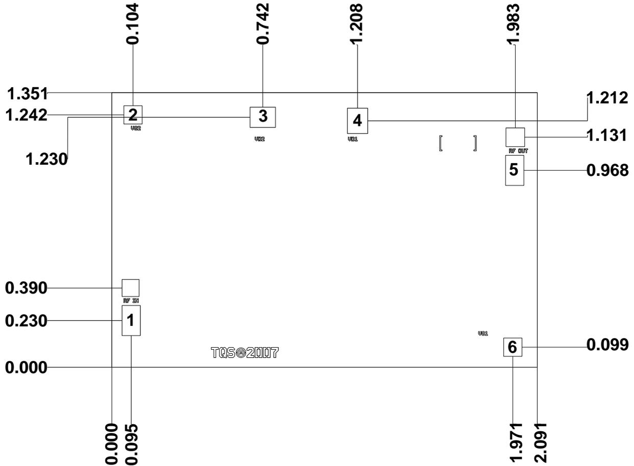
Unit: millimeters. Die thickness: 0.10, Die x, y size tolerance: +/- 0.050
