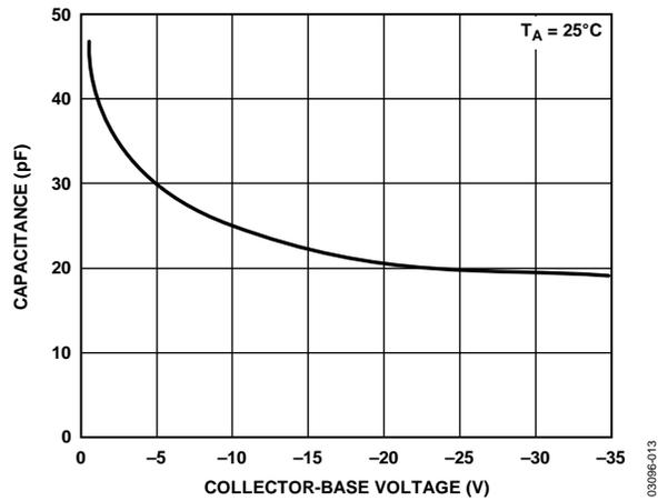
Figure 13. Collector to Base Capacitance vs.  $V_{CB}$
