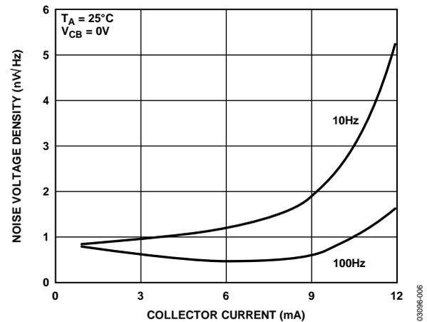
Figure 6. Noise Voltage Density vs. Collector Current
