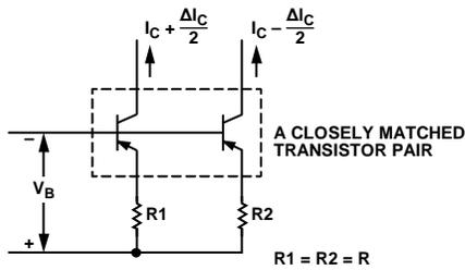
Figure 21. Current Matching Circuit
