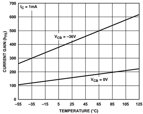
Figure 9. Current Gain ( $h_{FE}$ ) vs. Temperature
