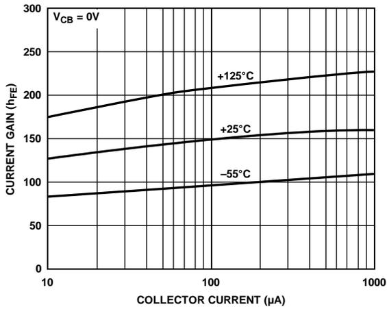
Figure 8. Current Gain ( $h_{FE}$ ) vs. Collector Current
