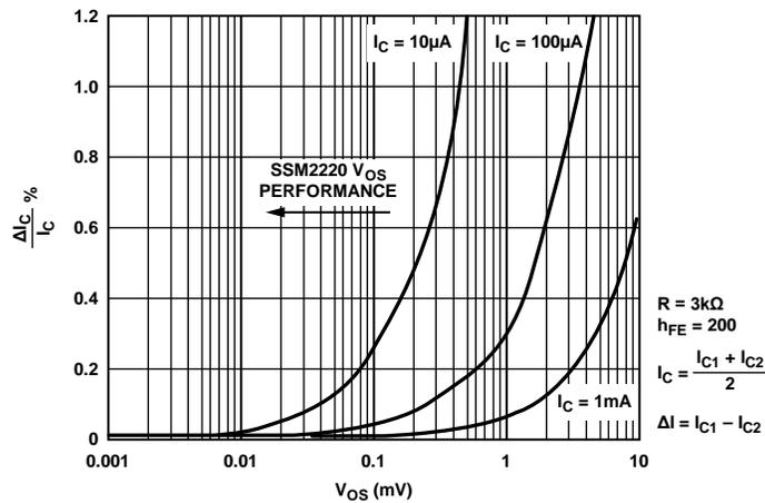
Figure 22. Current Matching Accuracy vs. Offset Voltage
