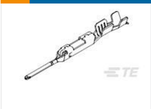
TE 产品编号1488208-1 0.64MM PIN CONTACT, CRIMP, 18-
