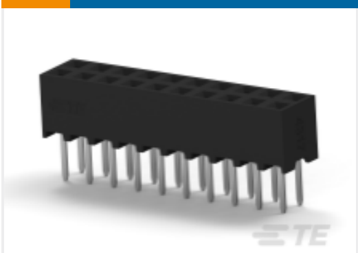
TE 产品编号2-2314822-0 20P,2MM,B-B,REC,DRVT,2.7,0.76AU,TB
