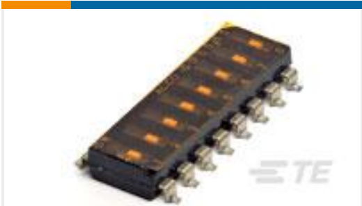
TE 产品编号1-1825006-9 GDS10S04=DIP SW,SLIDE,SMT
