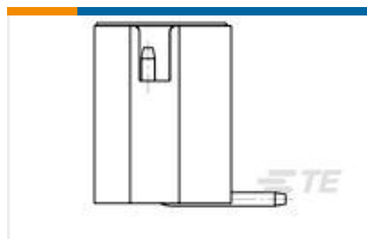
TE 产品编号1775470-2 HPI CONN., 2.0MM, V/T, SMT, 2P, 80U"
