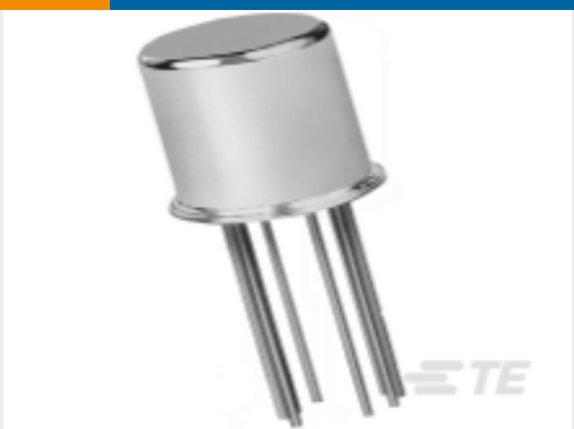
TE 产品编号4-1617520-4 1MACD-26=1MAD T05 1 POLE DIODE
