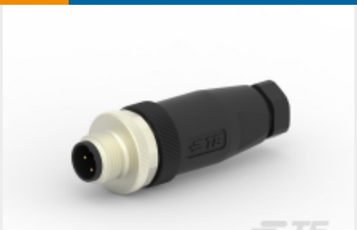
TE 产品编号T4111401031-000 M12,MALE,STRAIGHT,B CODE,3P, PG7,GOLD
