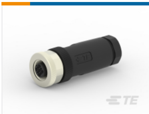
TE 产品编号T4110002051-000 M12,FEMALE,STRAIGHT,A CODE,5P, PG9,GOLD
