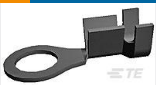
TE 产品编号160787-1 RING TONGUE IS 18-14 AWG .0840 X .940 BR
