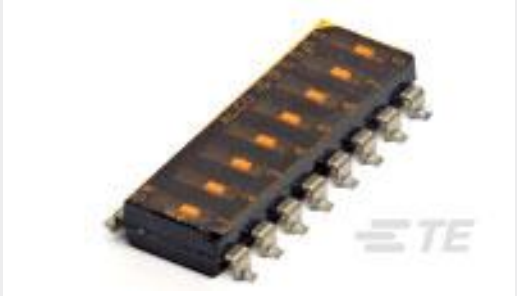
TE 产品编号1-1825006-9 GDS10S04=DIP SW,SLIDE,SMT
