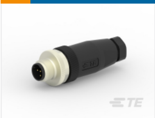
TE 产品编号T4111501051-000 M12,MALE,STRAIGHT,D CODE,5P, PG7,GOLD
