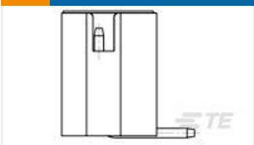
TE 产品编号1775470-9 HPI CONN., 2.0MM, V/T, SMT, 9P, 80U"
