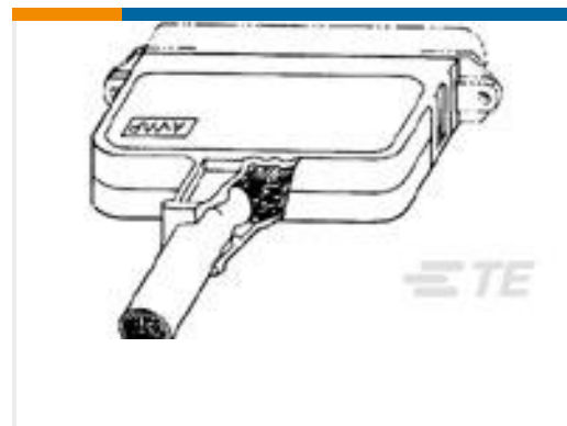
TE 产品编号1-552076-1 KIT, COVER, 180 DEG, 24 POS
