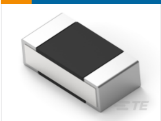
TE 产品编号5-2176306-9 RP 1E 0.1W 4K64 0.1% 25PPM 5K RL
