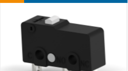
TE 产品编号2351450-1 SMINSA SW PPL 1.47N 5A/3A AC 3A DC SP
