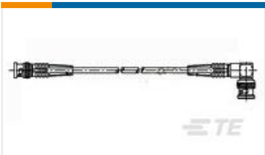
TE 产品编号1337772-3 50/OHM COAX BNC STR PLUG ELB P
