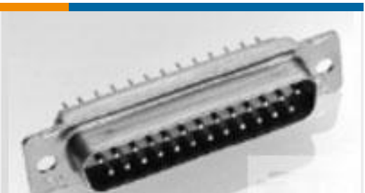
TE 产品编号204509-1 AMPLIMITE, ASY, PLUG, STD, 90, 5
