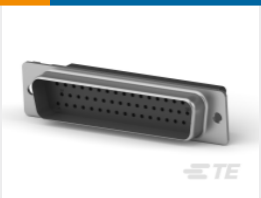
TE 产品编号1658641-3 D-Sub Crimp: Plug, Signal, 50 Posn, Pin Size 20, Shell Size 5
