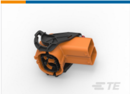
TE 产品编号1-2141154-1 2POS,8MM HV,REC HSG,90DEG,ASSY, SEALED
