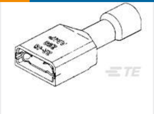
TE 产品编号3-520140-2 ULTRA-FAST 250 ASY REC 16-14 AWG TPBR
