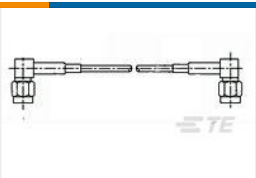
TE 产品编号1337812-3 50 OHM COAX SMA ELB PLUG ELB P
