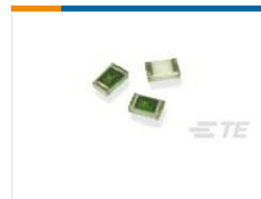
TE 产品编号1676153-1 RN 0805 10K 0.1% 10PPM CUT LENGTH
