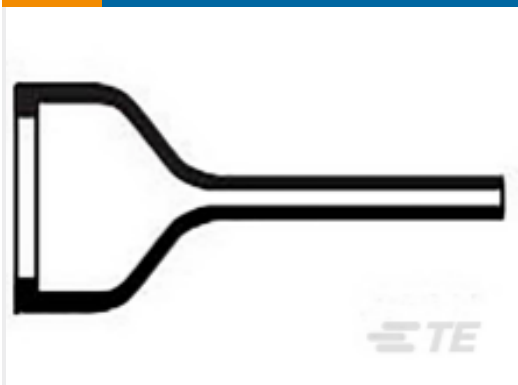
TE 产品编号808233-000 Heat Shrink Boots: Lipped, Straight
