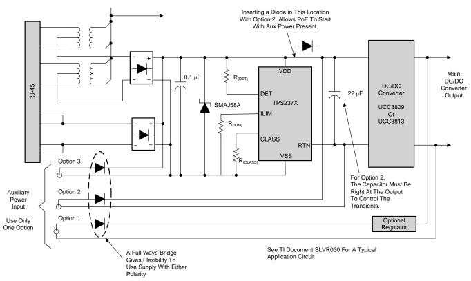
Figure 14. Auxiliary Power ORing
