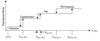
Figure 12. Threshold Voltages
