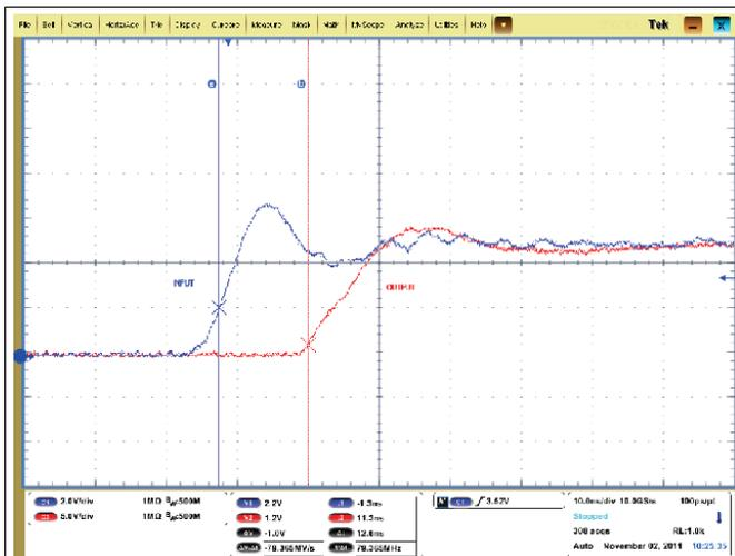
Figure 22. Turnon Propagation Delay
