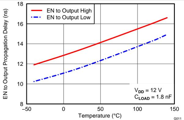
Figure 14. En to Output Propagation Delay vs Temperature
