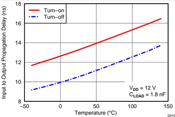
Figure 13. Input to Output Propagation Delay vs Temperature
