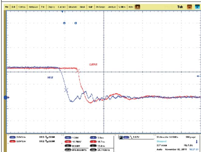
Figure 24. Turnoff Propagation Delay
