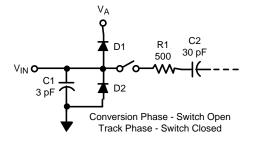
Figure 52. Equivalent Input Circuit
