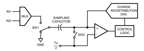
Figure 49. ADC082S101 in Hold Mode
