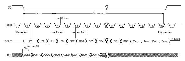
Figure 4. ADC082S101 Serial Timing Diagram
