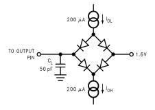
Figure 3. Timing Test Circuit
