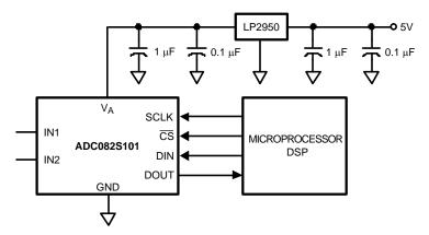
Figure 51. Typical Application Circuit
