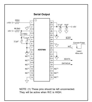
FIGURE 1b. Basic ±10V Operation with Serial Output.
