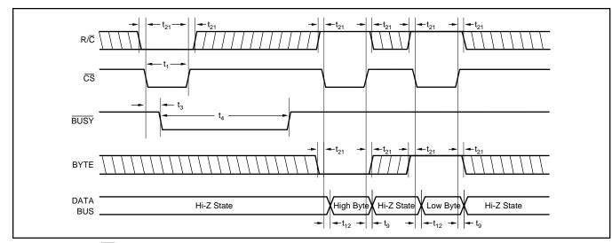
FIGURE 2. Conversion Timing with Parallel Output (CS and DATACLK tied LOW, EXT/INT tied HIGH).
