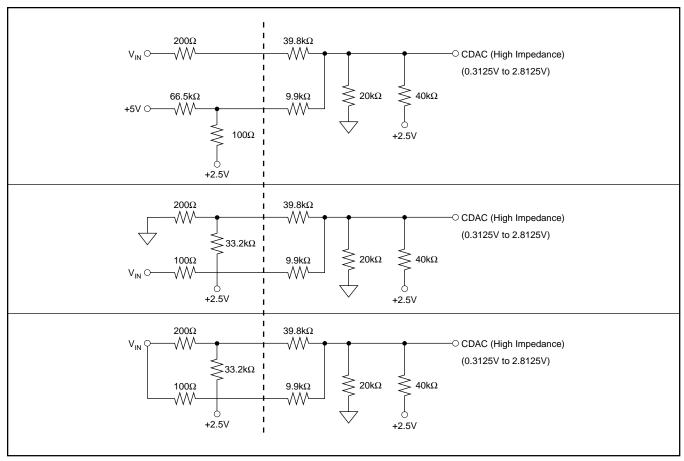
FIGURE 9. Circuit Diagrams Showing External and Internal Resistors.
