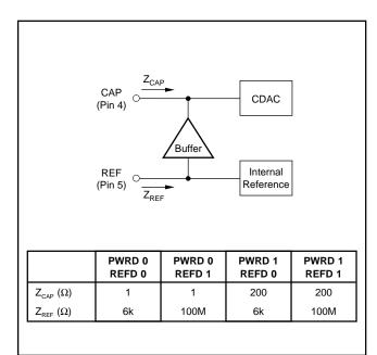
FIGURE 10. Characteristic Impedances of Internal Buffer.
