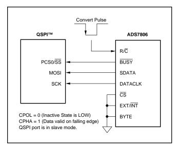
FIGURE 12. QSPI Interface to the ADS7806.
