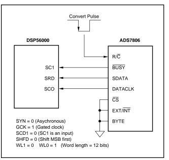
FIGURE 14. DSP56000 Interface to the ADS7806.
