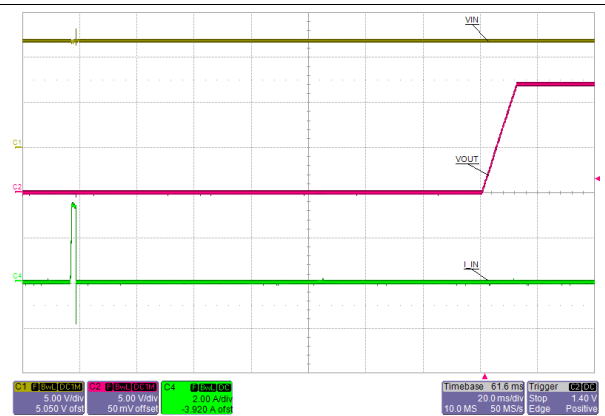
TPS25926x, V_{\text{VIN}} = 12\text{ V} , C_{\text{dVdT}} = 1\text{ nF}
