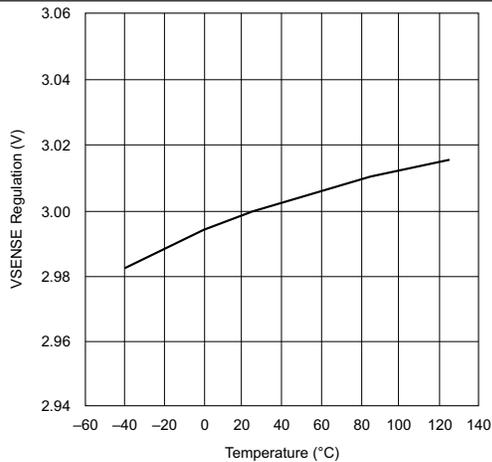
Figure 3. V<sub>VSENSE</sub> Regulation vs Junction Temperature
