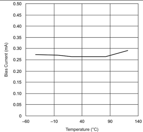
Figure 4. I<sub>VSENSE</sub> Bias Current vs Junction Temperature
