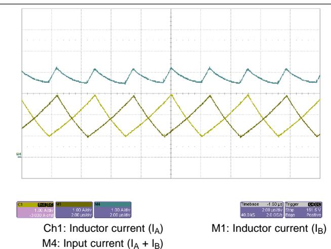
Figure 30. Typical Inductor and Input Ripple Currents
