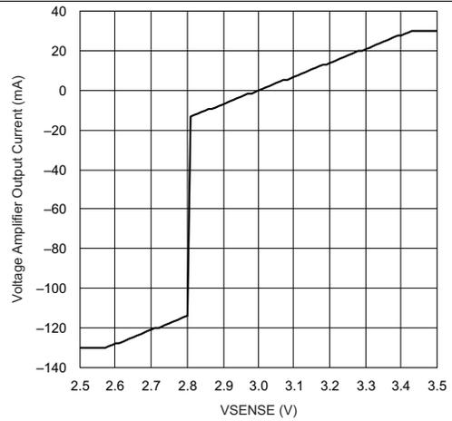
Figure 10. Voltage Amplifier Transfer Function vs  $V_{VSENSE}$
