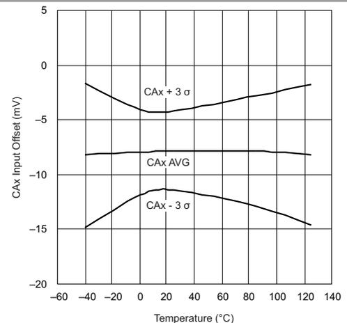
Figure 12. CAx Input Offset Voltage vs Junction Temperature
