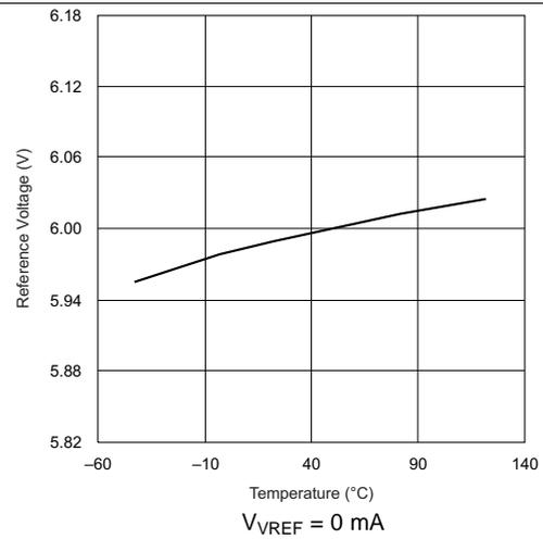
Figure 2. V<sub>VREF</sub> vs Junction Temperature
