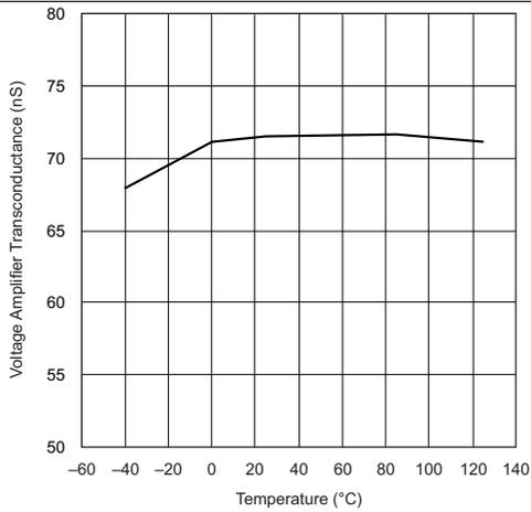
Figure 9. VAO, Voltage Amplifier Transconductance vs Junction Temperature
