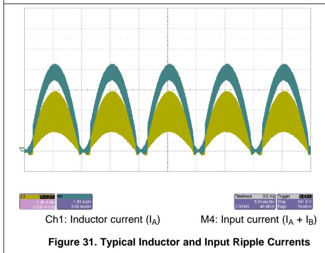
Figure 31. Typical Inductor and Input Ripple Currents
