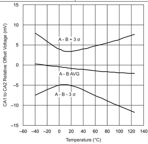
Figure 17. CA1 to CA2 Relative Offset vs Junction Temperature
