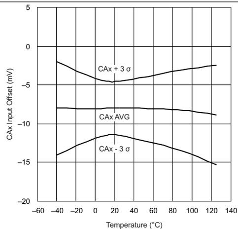
Figure 16. CAx Input Offset Voltage vs Junction Temperature
