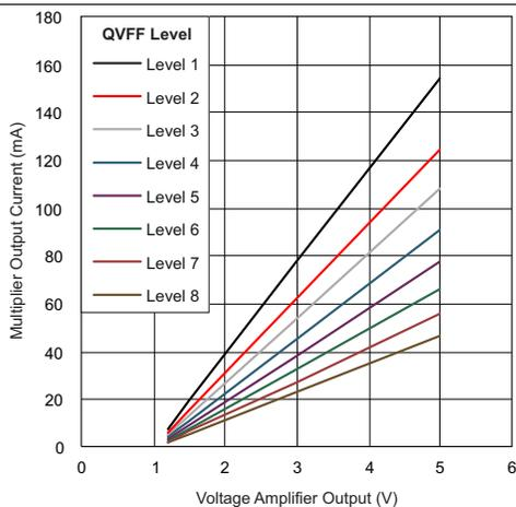
Figure 5. IMO, Multiplier Output Current vs V<sub>VAO</sub>
