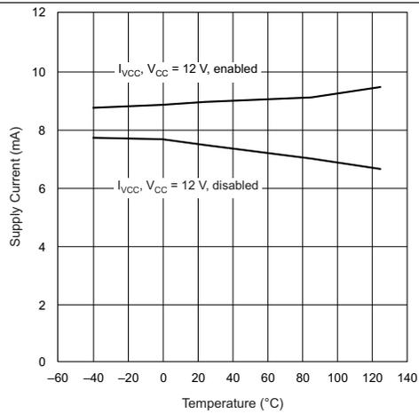
Figure 1. VCC Supply Current vs Junction Temperature
