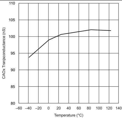
Figure 11. Current Amplifier Transconductance vs Junction Temperature
