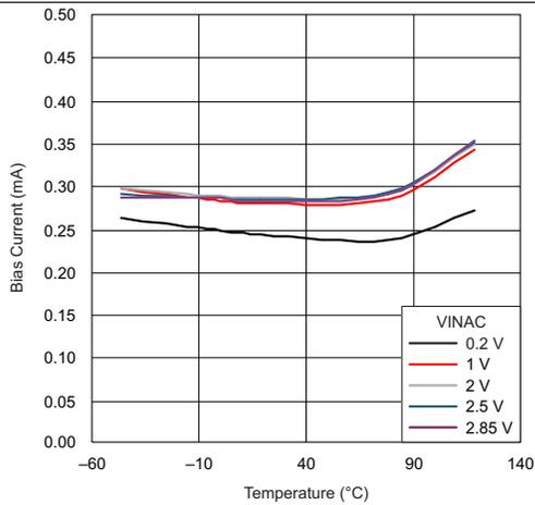
Figure 7.  $I_{VINAC}$  Bias Current vs Junction Temperature
