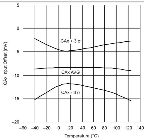
Figure 14. CAx Input Offset Voltage vs Junction Temperature
