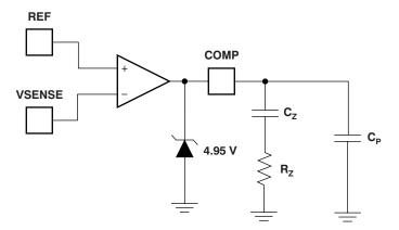
Figure 26. Typical Error Amplifier Compensation
