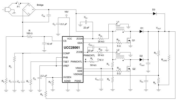
Figure 28. Typical Transition Mode Interleaved PFC Pre-Regulator
