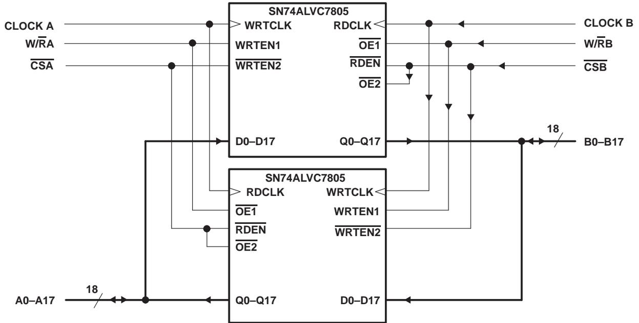
Figure 7. Bidirectional Configuration
