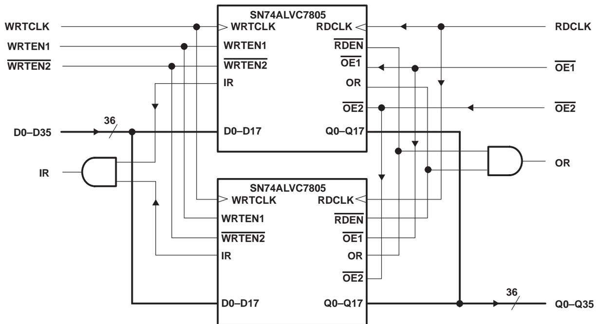
Figure 8. Word-Width Expansion: 256 × 36 Bits
