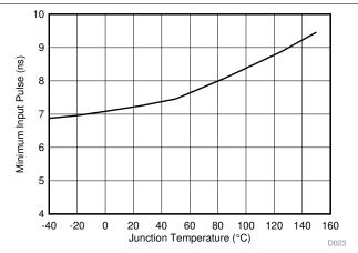
Figure 7-25. Minimum Pulse that Changes Output
