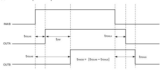
Figure 8-3. Delay Matching and Pulse Width Distortion
