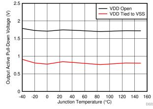
Figure 7-24. OUTPUT Active Pulldown Voltage
