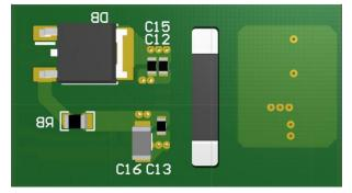
Figure 12-5. 3-D PCB Bottom View
