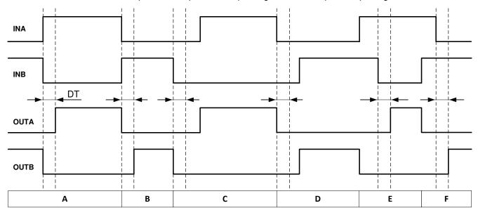
Figure 9-4. Input and Output Logic Relationship with Input Signals
