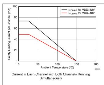
Figure 7-2. Thermal Derating Curve for Limiting **Current Per VDE**
