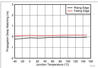
Figure 7-20. Propagation Delay Matching, Rising and Falling Edge
