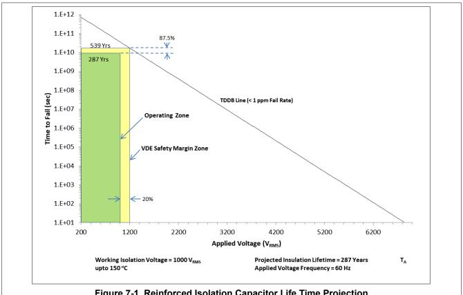
Figure 7-1. Reinforced Isolation Capacitor Life Time Projection
