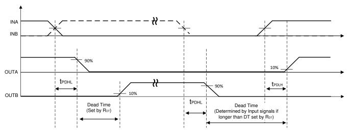
Figure 8-6. Dead Time Switching Parameters
