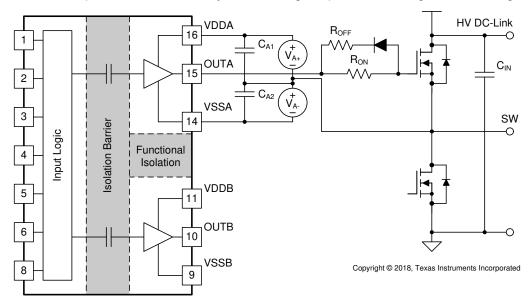
Figure 10-3. Negative Bias with Two Iso-Bias Power Supplies
