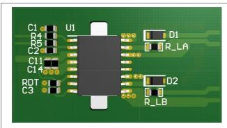
Figure 12-4. 3-D PCB Top View
