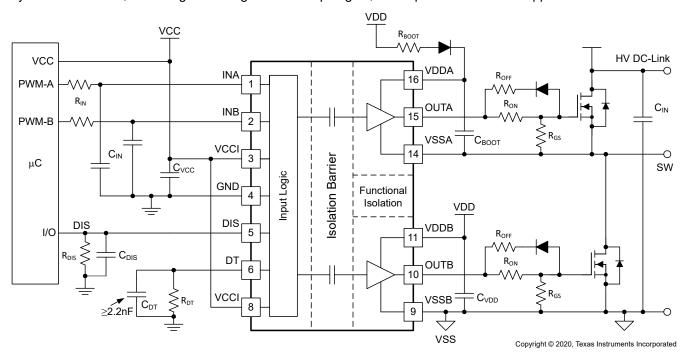
Figure 10-1. Typical Application Schematic
