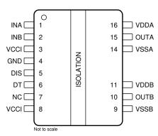
Figure 6-1. DWK Package 14-Pin SOIC Top View
