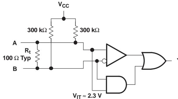
**Figure 18. Open-Circuit Fail Safe of the LVDS Receiver**
