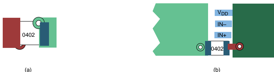
Figure 22. Typical Decoupling Capacitor Layouts
