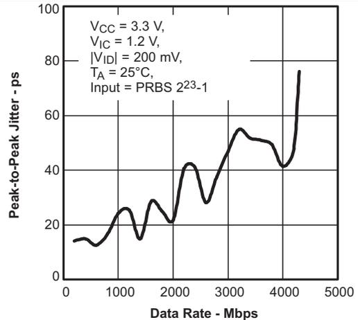
Figure 24. SN65LVDS101 Peak-to-Peak Jitter vs Data Rate
