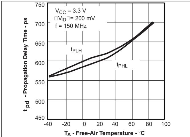
Figure 7. SN65LVDS101 Propagation Delay Time vs Free-Air Temperature
