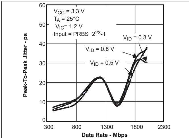
Figure 13. SN65LVDS100 Peak-to-Peak Jitter vs Data Rate
