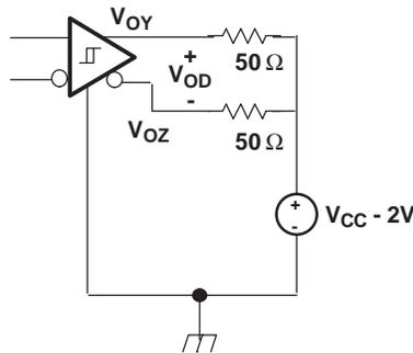
Figure 39. Typical Termination for LVPECL Output Driver (SN65LVDS101)
