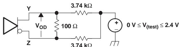
Figure 31. SN65LVDSx100 Differential Output Voltage (V<sub>OD</sub>) Test Circuit
