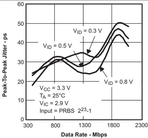
Figure 19. SN65LVDS101 Peak-to-Peak Jitter vs Data Rate
