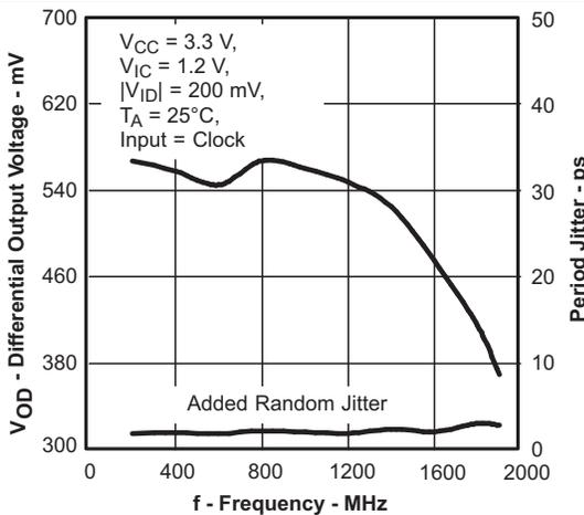
Figure 23. SN65LVDS101 Differential Output Voltage vs Frequency
