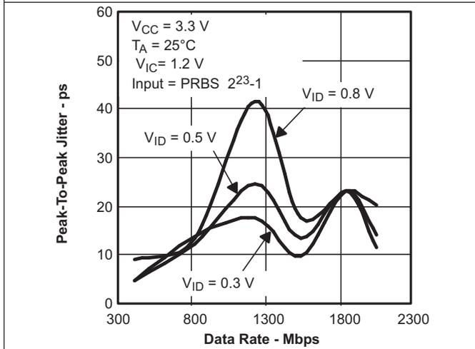
Figure 15. SN65LVDS101 Peak-to-Peak Jitter vs Data Rate
