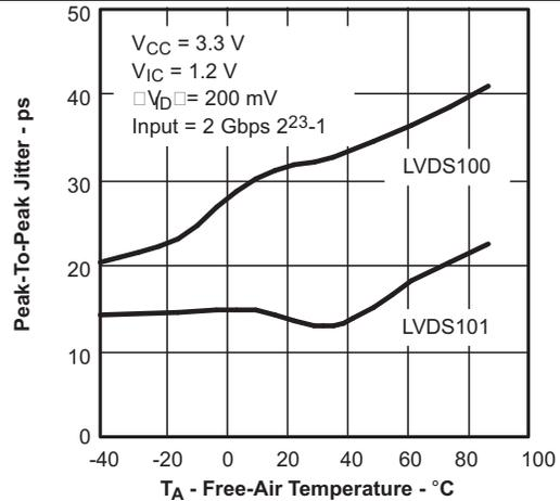
Figure 20. SN65LVDS100 Peak-to-Peak Jitter vs Free-Air Temperature
