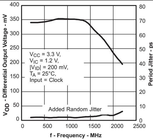
Figure 21. SN65LVDS100 Differential Output Voltage vs Frequency
