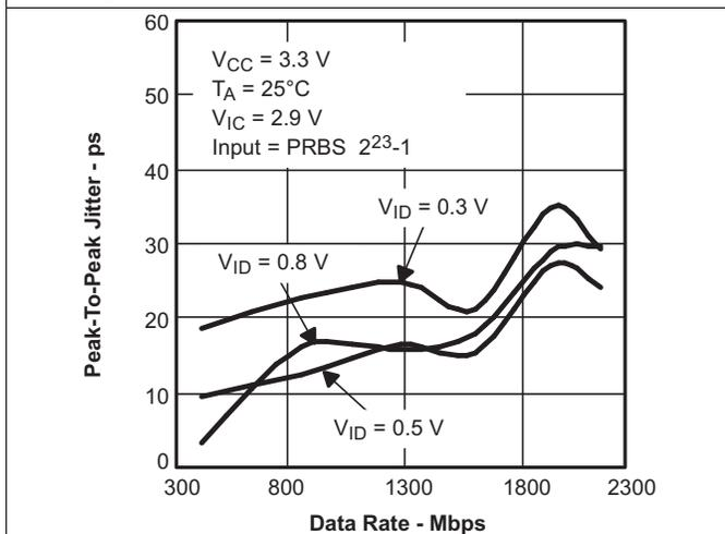
Figure 17. SN65LVDS100 Peak-to-Peak Jitter vs Data Rate
