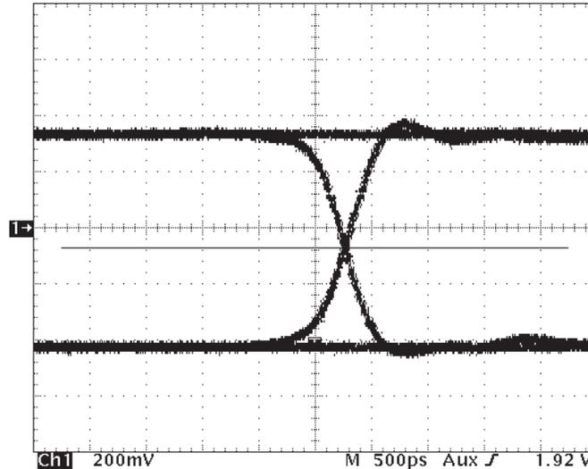
**Figure 37. Receiver Input Eye Pattern with External Failsafe**
