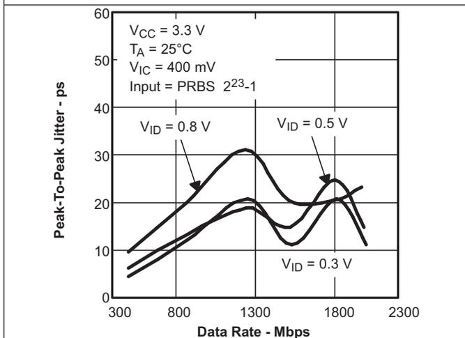
Figure 11. SN65LVDS101 Peak-to-Peak Jitter vs Data Rate
