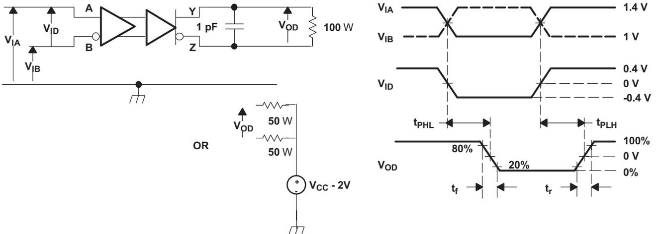
NOTE: All input pulses are supplied by a generator having the following characteristics:  $t_r$  or  $t_f \leq 0.25$  ns, pulse repetition rate (PRR) = 50 Mpps, pulse width =  $10 \pm 0.2$  ns.  $C_L$  includes instrumentation and fixture capacitance within 0.06 mm of the device under test. Measurement equipment provides a bandwidth of 5 GHz minimum.
