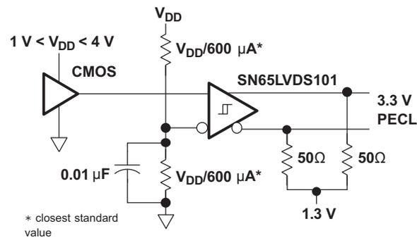
**Figure 49. Single-Ended CMOS to 3.3-V PECL Translation**
