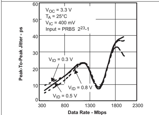
Figure 9. SN65LVDS100 Peak-to-Peak Jitter vs Data Rate
