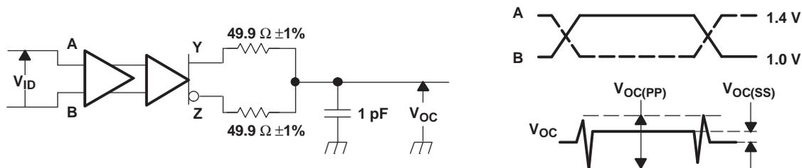
NOTE: All input pulses are supplied by a generator having the following characteristics:  $t_r$  or  $t_f \leq 0.25$  ns, pulse repetition rate (PRR) = 0.5 Mpps, pulse width =  $500 \pm 10$  ns.  $C_L$  includes instrumentation and fixture capacitance within 0.06 mm of the device under test. The measurement of  $V_{OC(PP)}$  is made on test equipment with a -3 dB bandwidth of at least 300 MHz.
