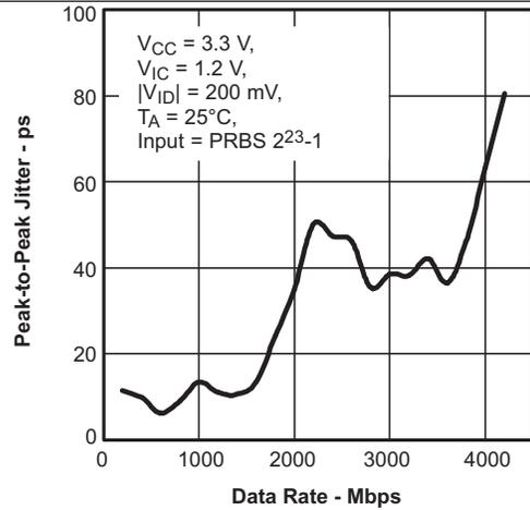
Figure 22. SN65LVDS100 Peak-to-Peak Jitter vs Data Rate
