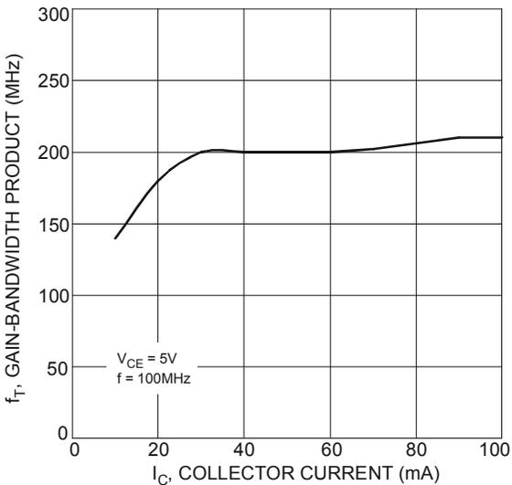
Fig. 7 Typical Gain-Bandwidth Product vs. Collector Current
