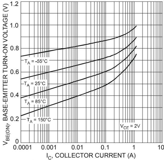
Fig. 3 Typical Base-Emitter Turn-On Voltage vs. Collector Current
