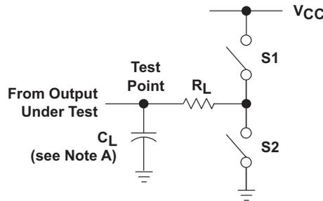
Figure 2. Load Circuit
