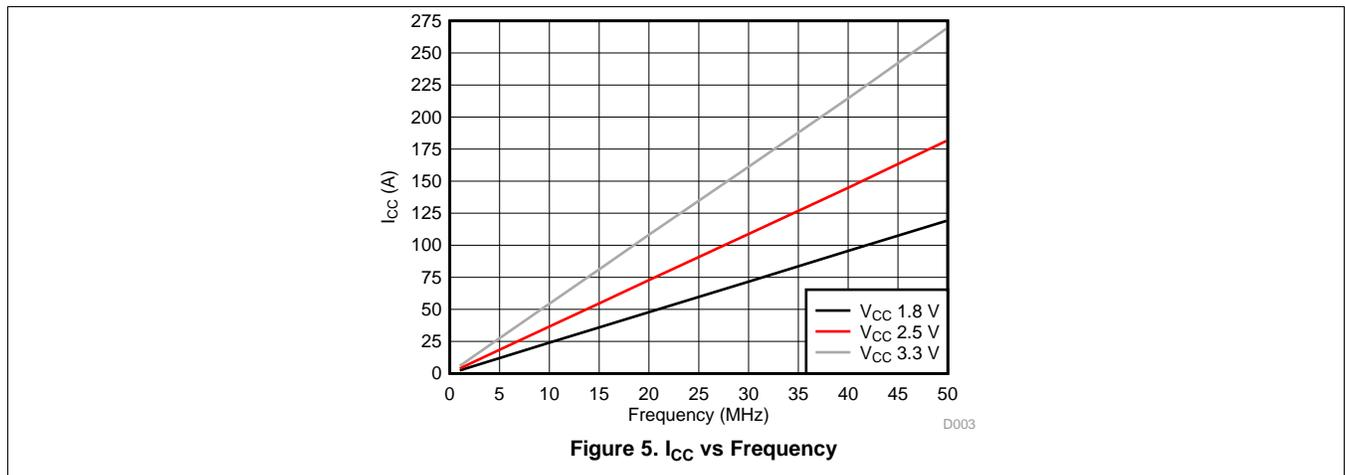
Figure 5. I<sub>CC</sub> vs Frequency
