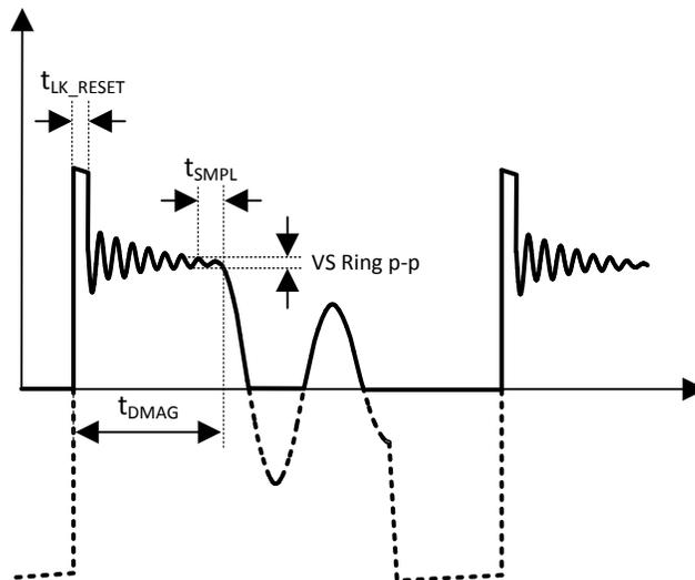
Figure 22. VS Voltage
