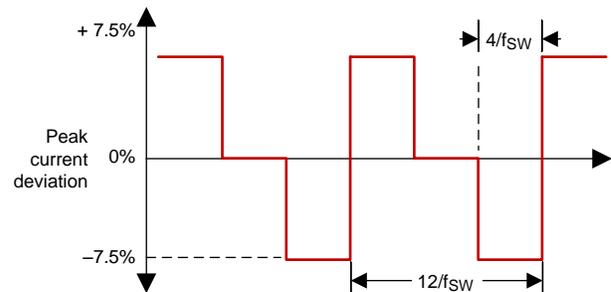
**Figure 32. EMI Dithering During CC Mode Operation**
