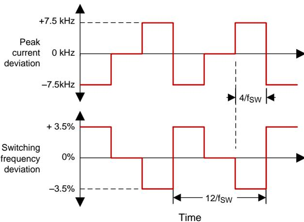
**Figure 31. EMI Dithering During CV Mode Operation**
