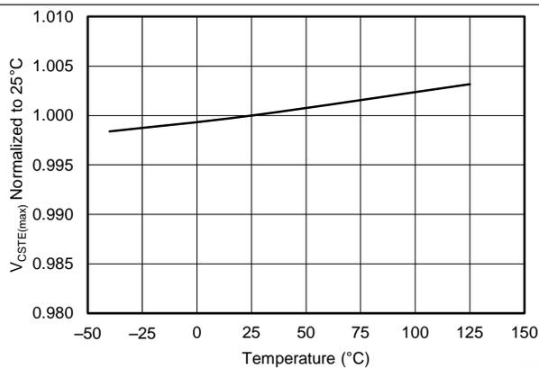
Figure 6. UCC28910  $V_{CSTE(max)}$  vs Temperature
