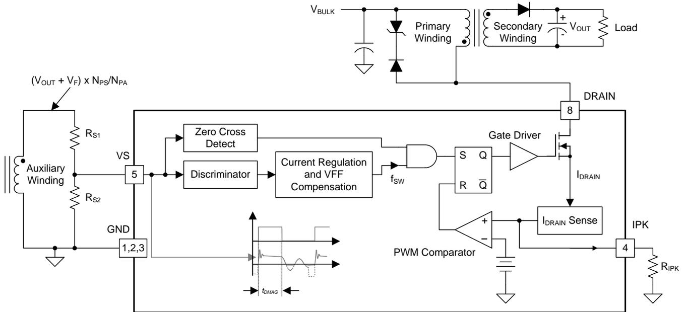
**Figure 25. Output Current Control Loop Block Diagram**
