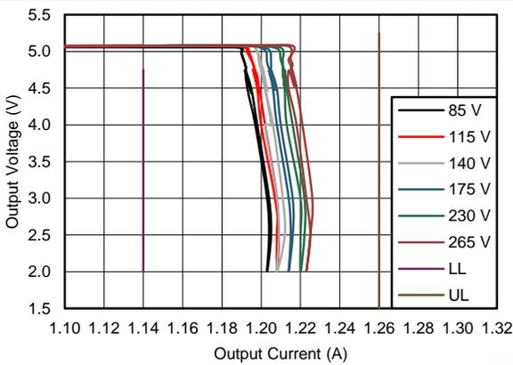
Figure 43. Output V-I Characteristic Output Voltage Regulation
