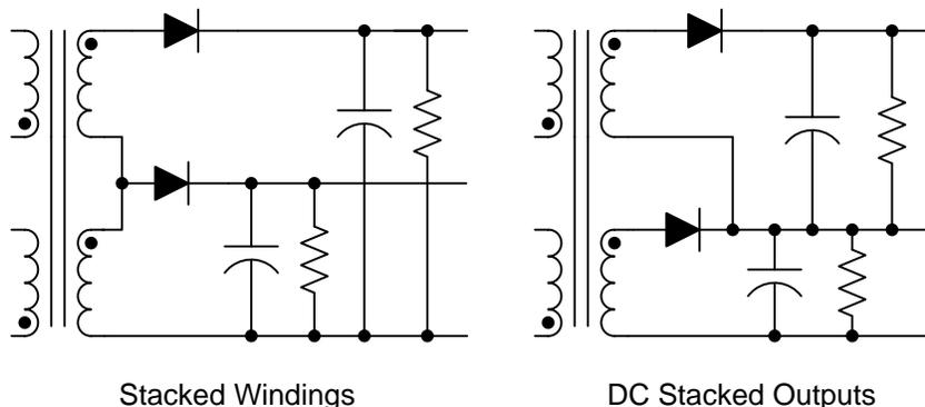
**Figure 51. Stacked Windings and DC Stacked Outputs**
