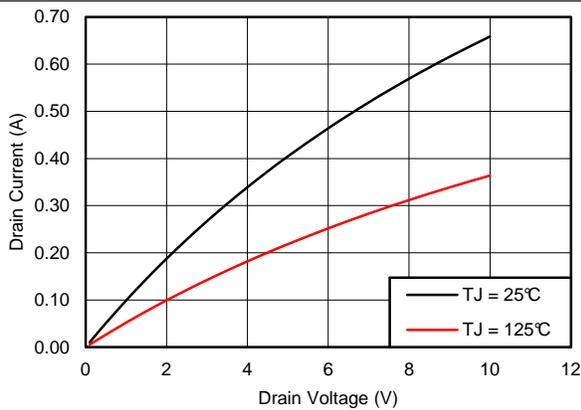
Figure 4. UCC28910 Drain Current vs Drain Voltage
