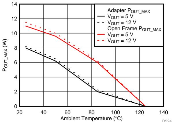
**Figure 38. 90 V<sub>RMS</sub>, 264 V<sub>RMS</sub> Input Voltage Range, (maximum output power vs ambient temperature of UCC28911)**
