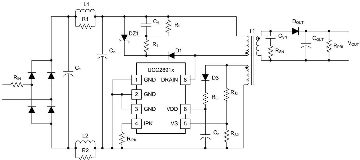
**Figure 35. Standard Flyback Converter Based on UCC2891x**
