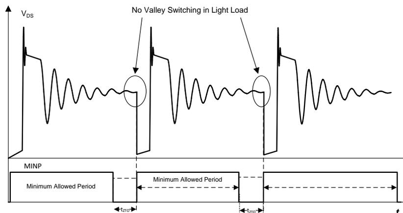
Figure 29. Valley Switching Disable at Light Load
