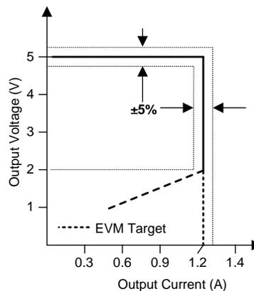
Figure 33. Target Output V-I Characteristic
