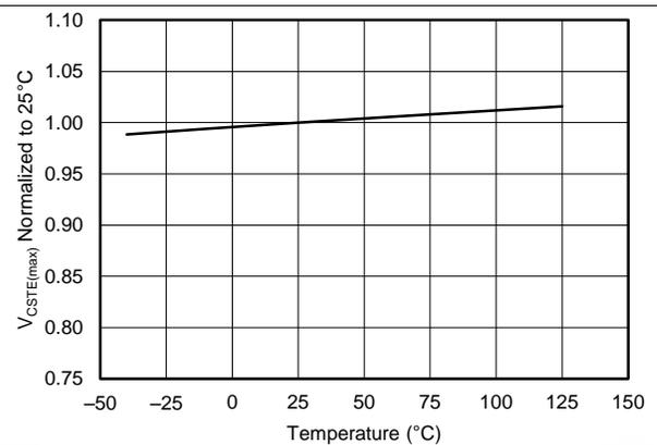
Figure 7. UCC28911  $V_{CSTE(max)}$  vs Temperature
