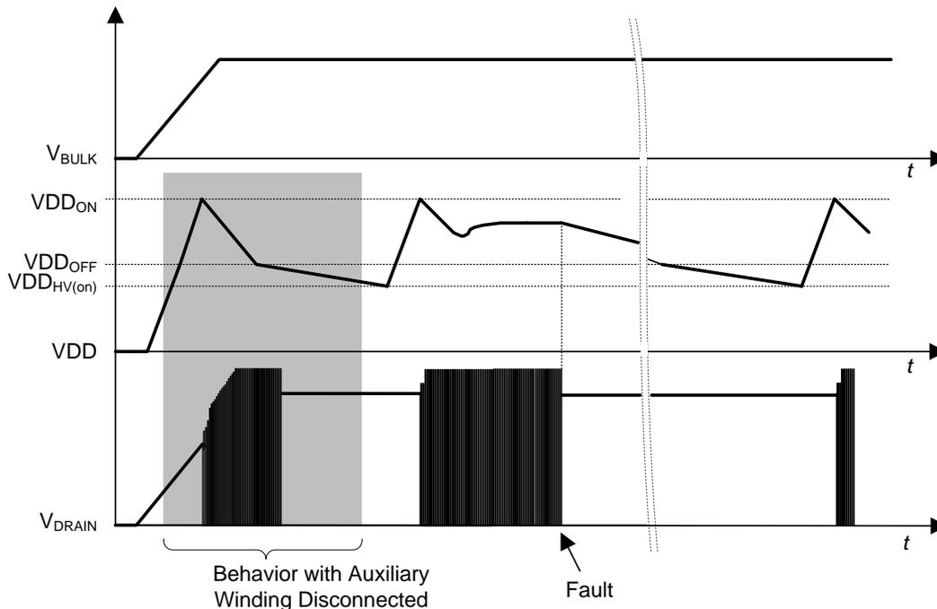
**Figure 30. Start Up and Auto Re-Start Operation**
