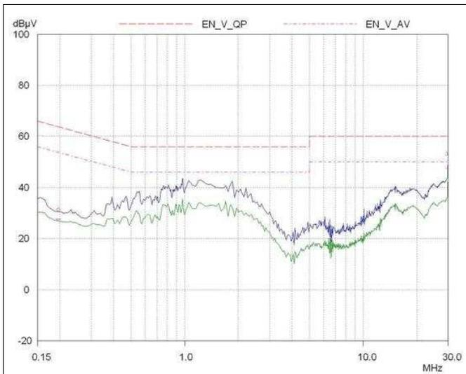
**Figure 47. EMI Test Results per EN55022, Class B. 115 V<sub>AC</sub> Input**
