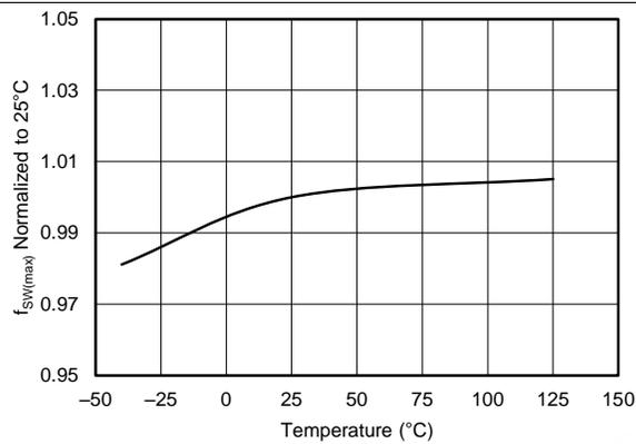
Figure 12.  $f_{SW(max)}$  vs Temperature
