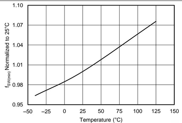
Figure 13.  $f_{SW(min)}$  vs Temperature
