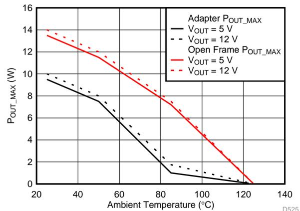
**Figure 39. 180 V<sub>RMS</sub>, 264 V<sub>RMS</sub> Input Voltage Range, (maximum output power vs ambient temperature of UCC28911)**
