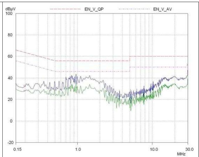
**Figure 48. EMI Test Results per EN55022, Class B. 230-V<sub>AC</sub> Input**
