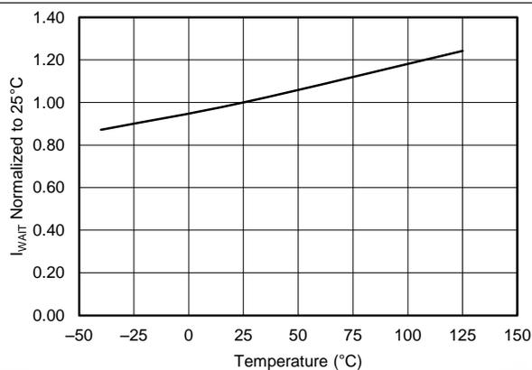
Figure 18.  $I_{WAIT}$  vs Temperature
