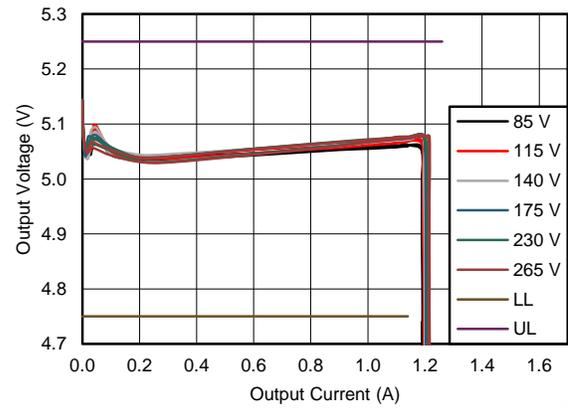
Figure 42. Output V-I Characteristic Output Current Regulation
