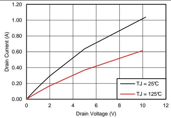
Figure 5. UCC28911  $D_{RAIN}$  Current vs  $D_{RAIN}$  Voltage
