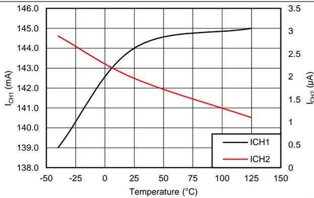
Figure 16.  $I_{CH1}$  and  $I_{CH2}$  vs Temperature
