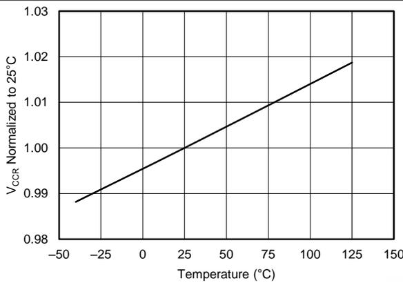
Figure 10. UCC28910  $V_{CCR}$  vs Temperature
