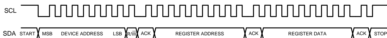
Figure 26. Example I 2 C Write Cycle
