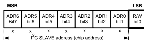
Figure 18. I²C Chip Address
