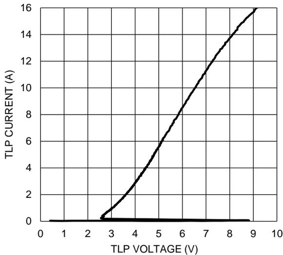
Figure 5 TLP Curve (t<sub>p</sub> = 100ns)
