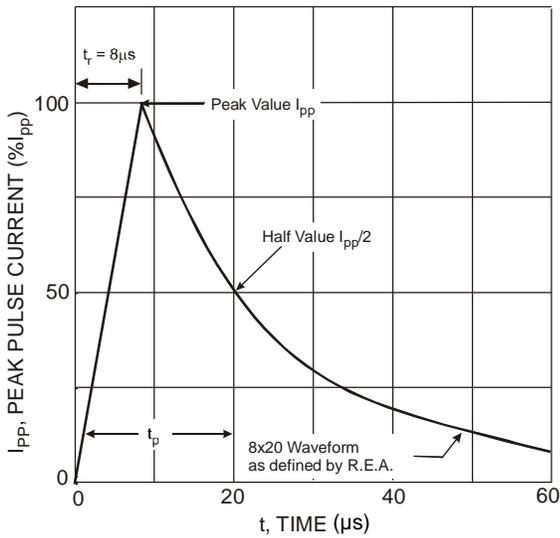
Figure 3 Pulse Waveform
