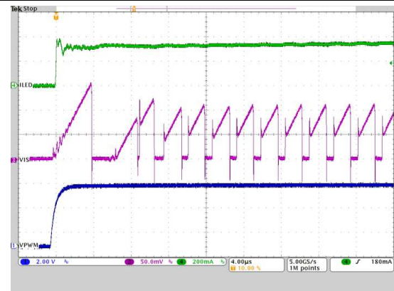
Ch1: External PWM input voltage; Ch3: Switch sense current resistor voltage; Ch4: LED current; Time: 4 \mu s/div
