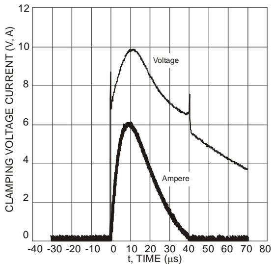
Figure 5 Waveform of Clamping Voltage, Current vs. Time (8/20µs, I/O to V<sub>SS</sub>)
