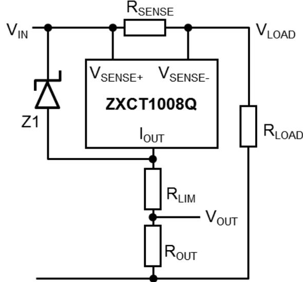
Figure 1. ZXCT1008Q with Additional Current Limiting Resistor R<sub>LIM</sub> and Zener Z1
