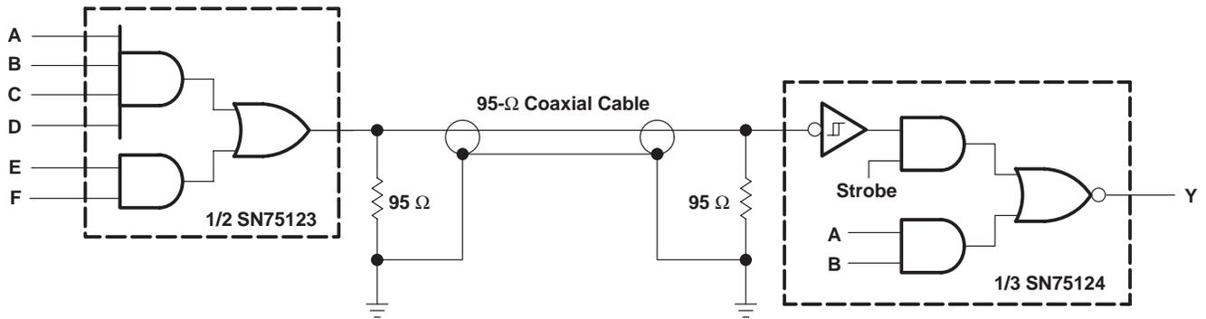
Figure 3. Unbalanced Line Communication Using SN75123 and SN75124
