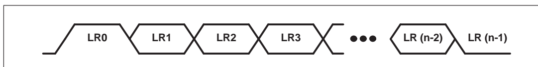
Figure 25. PINT (PHY Interrupt) Stream
