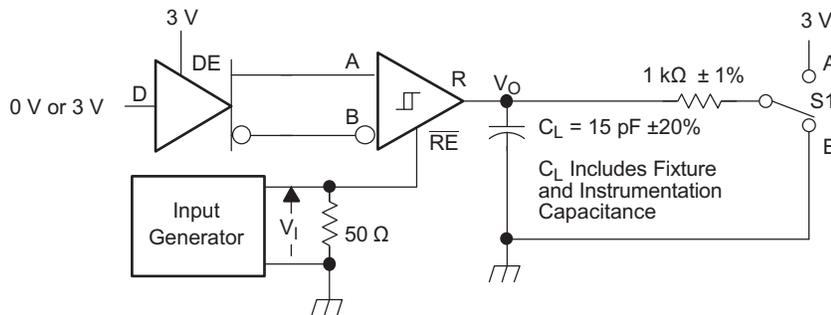
Generator: PRR = 500 kHz, 50% Duty Cycle,  $t_r < 6$  ns,  $t_f < 6$  ns,  $Z_o = 50 \Omega$
